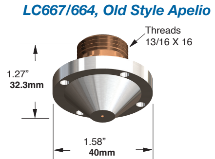
Nozzle (Clean Cut) 71102000 1.5mm 71102000-1.75 1.75mm 71101999 2.0mm 71101999-2.5 2.5mm
