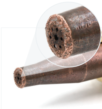
Original worn out tip.
