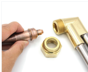
Remove standard tip nut and worn out oxy-fuel tip.
